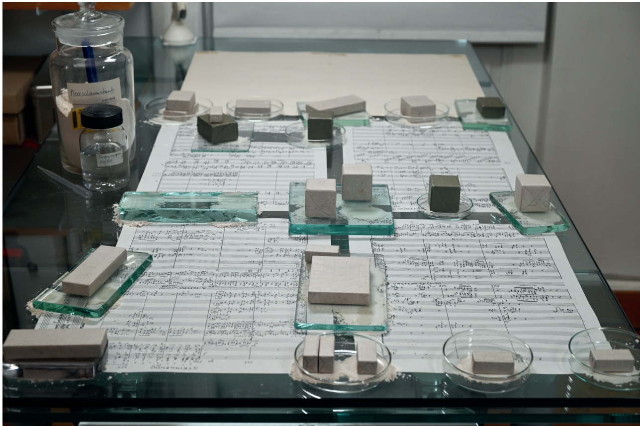
Figure 11 Removal of oily components with sepiolite poultices
