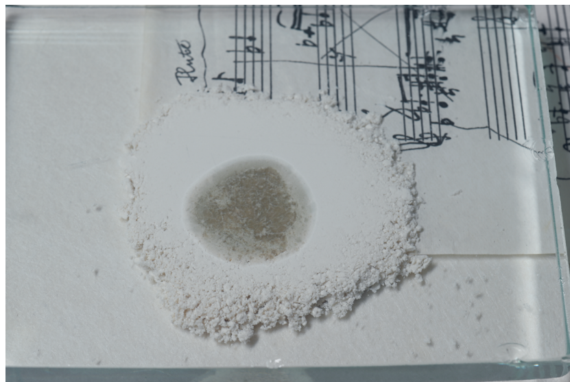
Figure 8 Sketch, sepiolite poultice with white spirit
